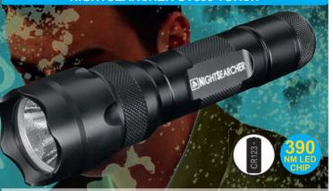
• 1 W High Power UV LED with Wavelength 390 - 395nm Lightweight and compact flashlight 1W LED emitting a powerful Ultra Violet Beam. Designed specifically for forensic applications and crime investigation. Manufactured in durable aluminium casing it is water and shock resistant. 2 CR123A batteries (not included) Run Tim 3.5 hrs / 6hrs. Designed for Forensic & SOC applications. Length 132mm Head Dia 33.5mm. Weight 144g (inc. batteries)
